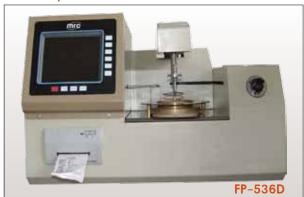
The instrument is designed and made as per the National Standard of People' Republic of China GB/T3536–2008 "Test Methods for Flash and Fire Point of Petroleum Products (Cleveland Open Cup Methods)". it is suitable to determine flash point and fire point of petroleum products having a flash point higher than 79 t, excepting fuel oils.
