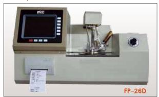
This instrument is suitable to the standards of GB/ T261 . It uses the closed cup to test the flash point of liquid. Reference standard: 1502791, ASTMD93, IP34
