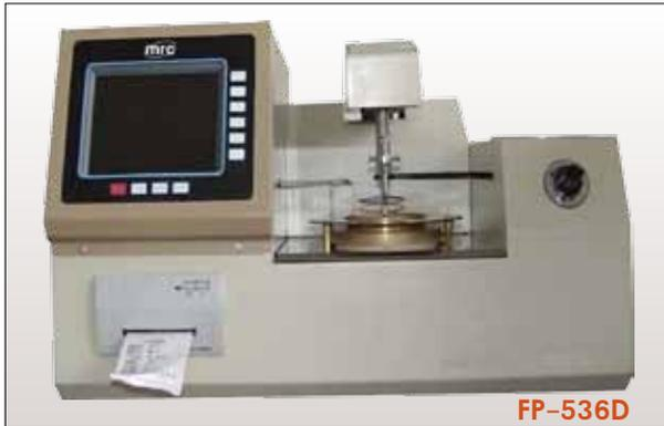
The instrument is designed and made as per the National Standard of People's Republic of China GB/T3536-2008 "Test Methods for Flash and Fire Point of Petroleum Products (Cleveland Open Cup Methods)". It is suitable to determine flash point and fire point of petroleum products having a flash point higher than 79 °C, excepting fuel oils.
