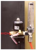
Connect the nitrogen supplying gas to the back solenoid with quick fit 8mm tube and make sure the gas pressure will not exceed 7 Kg/cm<sup>2</sup>
