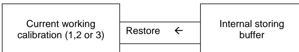
The current calibration is replaced with the calibration from the internal buffer and the analyzer starts working with it. The content of the internal buffer is not changed.
