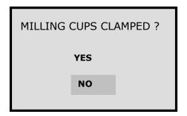
The software of the PM400 is set up in such a way that when operating the start button the following display appears, in which clamping of the milling cups has to be confirmed before every machine start up.
