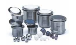
**RETSCH Planetary Ball Mills** are used for the pulverization of **soft, fibrous, hard and brittle ma-terials**. They achieve a very high final fineness down to the submicron range. The feed size depends on the mill and can be as large as 10 mm. If the sample feed size is larger than this then the sample must first undergo preliminary size reduction.
