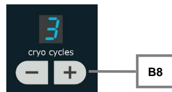
Fig. 35: Setting the grinding cycles
