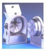
The material sample is crushed by two milling discs coarsely meshed on the inside working against one another in a milling space sealed against dust from the outside. One of these is driven by a powerful and slow moving gear motor.
