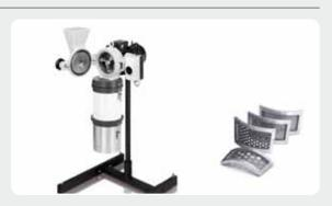
The rotor mill series includes ultra centrifugal mills, rotor beater mills and cross beater mills. Depending on the particular instrument they are suitable for the preliminary and fine size reduction of soft, fibrous and also hard materials. A final fineness of down to 40 µm can often be achieved in the first working step. The maximum feed size depends on the mill and ranges from 10 to 15 mm. Material which is larger than this must first undergo preliminary size reduction.
