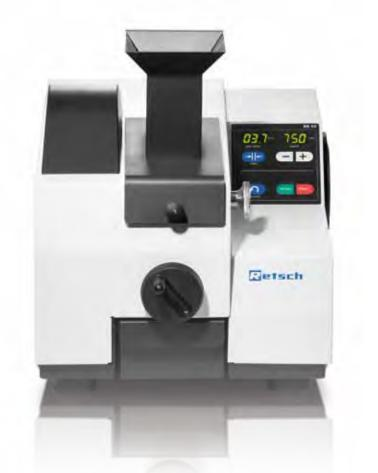
The BB 50 is designed for a very efficient and convenient size reduction process. The **variable speed** can be set between **550 and 950 min-**<sup>1</sup> to adapt the crushing process to sample requirements. The possibility to **reverse the rotating direction** is helpful if too much sample material has been fed to the crusher causing it to block. The simple push of a button restarts the process. There is no need to empty the crushing chamber manually.
