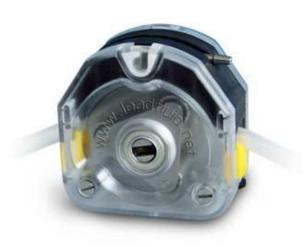
KZ25 pump head is suitable for the big flow transmission, up to 6800mL/min, can load various tubing. Replacing tubing only wastes several seconds, easy to operate. can be mounted in tandem(up to 2). The rollers adopt 304 stainless steel, the shell adopts transparent PC material, moderate intensity, it is convenient for observing the internal work situation of pump head. The top press block adopts PPS material which is resistant to high temperature and corrosion.
