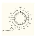
Turning timer knob allows the M100 to run for 1 min to 60 minutes clockwise
