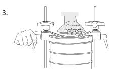
The side handle levers can be set vertically downwards by pressing on the Red button and pulling the handle outwards to release. Turn the handle to a safe, convenient angle downwards and release to engage the teeth. Screw the
