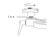
Ensure that the clamping handwheels at the top are loose and the locking assemblies are fully pushed down. There should be a 5mm gap between the large plain washer and the face of the handwheel.
