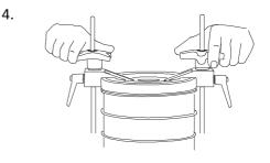
down simultaneously to ensure the clamping plate is square. Continue until the handwheels are tight against the internal stop. Hand tightness must be exerted so that the assembly does not loosen during vibration.
