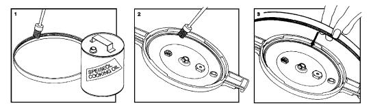
WE RECOMMEND THE CERTOCLAV SERVICE SET **ART. No.: 1250499**. It contains all spares which are under wear and tear and have to be replaced. (Lid gasket 1260404, Gasket for Manometer + Steam release cock 1250451, Gasket for valve 1250433, Steam release valve 1250242)
