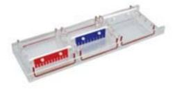
CASTING TIP Regardless of the casting method, ensure leak-free casting by lining the casting unit with agarose and allowing it to set before pouring the remainder of the hand-hot agarose mixture i.e. at approx. 50°C
