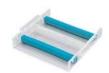
CASTING TIP Regardless of the casting method, ensure leak-free casting by lining the casting unit with agarose and allowing it to set before pouring the remainder of the hand-hot agarose mixture i.e. at approx.
