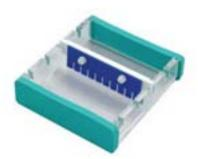
**HU10-CU** - silicone gaskets, seated in the groove of each casting tray, form a leak-free seal against the walls of the casting unit, allowing 3 gels to be cast simultaneously
