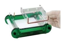
**HU10-SS** - 10cm long Scie-Plas Super-Seals offer total versatility in casting, allowing the gel length to be tailored to each user's personal requirements
