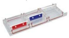
TECHNICAL TIP | Gasket too tight or loose? Simply remove the gaskets from the ends of the gel trays and refit into the groove. Refit with the gasket protruding slightly from the ends if the gel tray was too tight or with the gasket fitted below the top edges if the gasket was too loose.
