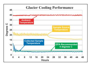
Glacier's exclusive temperature control technology accurately preserves samples at  $3 \,^{\circ}$  C – even under the difficult conditions shown here (40  $^{\circ}$  C ambient, 20  $^{\circ}$  C sample temperature).
